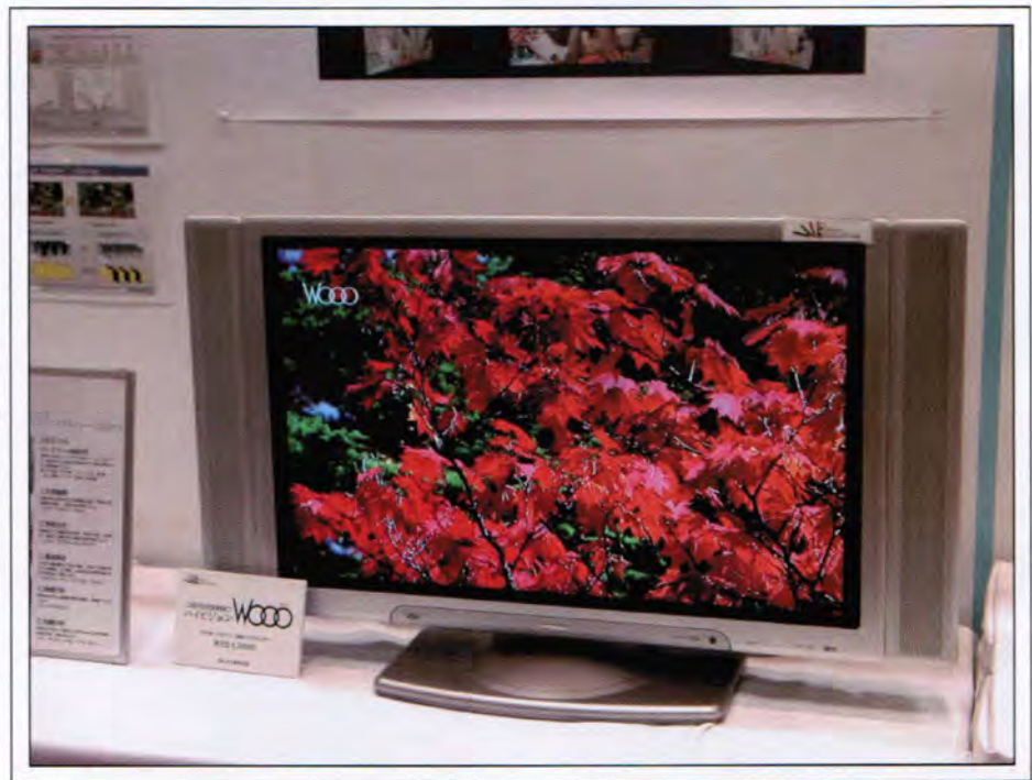
Fig. 3: At the low-keyed exhibition, Hitachi showed its 32-in. WOOO LCD TV based on its black-data-insertion approach, which produces pictures remarkably free of motion smear.
